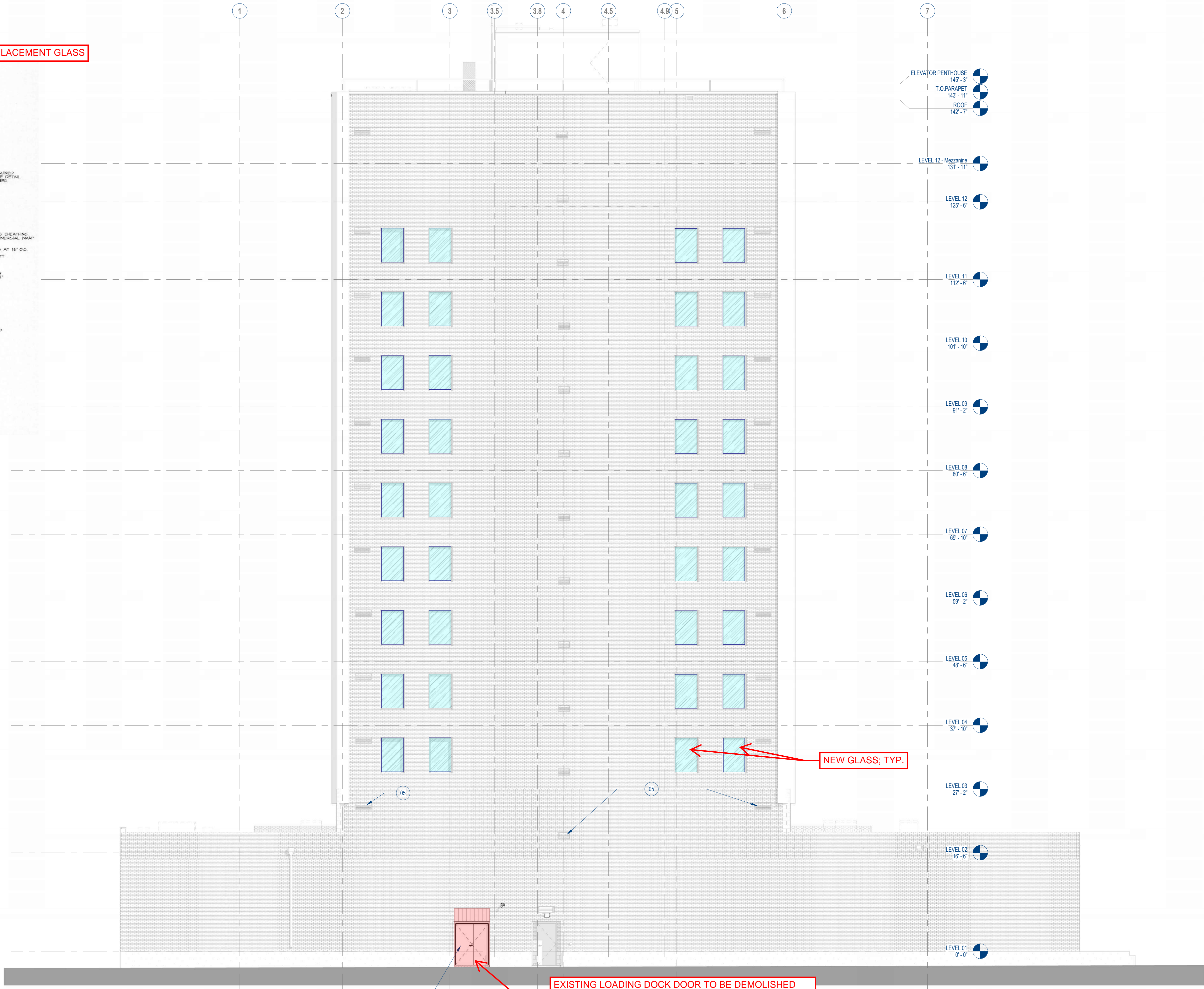
EXISTING LOADING DOCK DOOR TO BE DEMOLISHED AND REPLACED WITH WITH DOUBLE DOOR, AT LOWER ALLEY ELEVATION. AREA ABOVE DOOR TO BE INFILLED WITH PRE-FINISHED RIBBED METAL PANELS.
