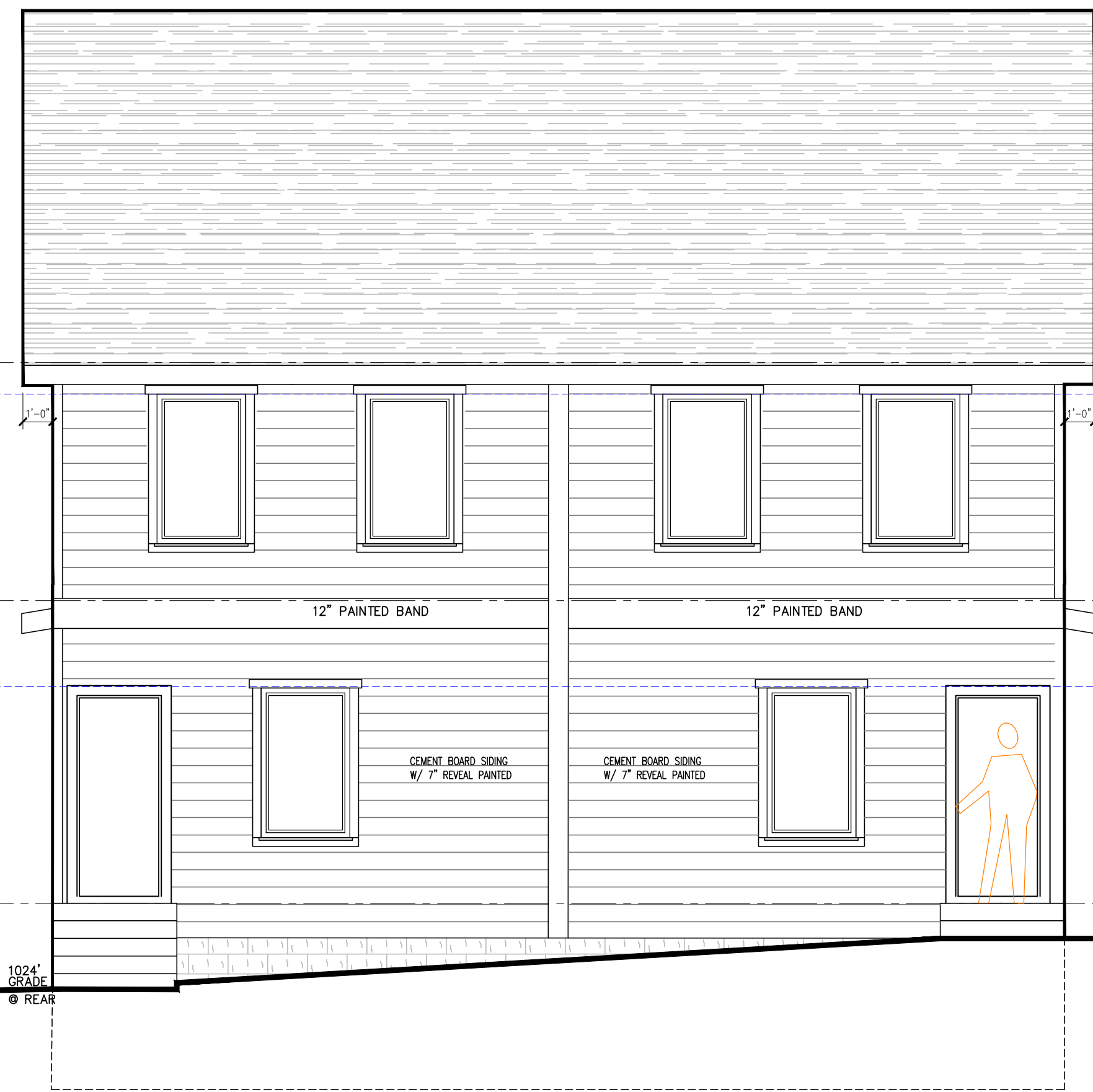
REAR ELEVATION UNIT "B" UNIT "A" 1/4" = 1'-0"
