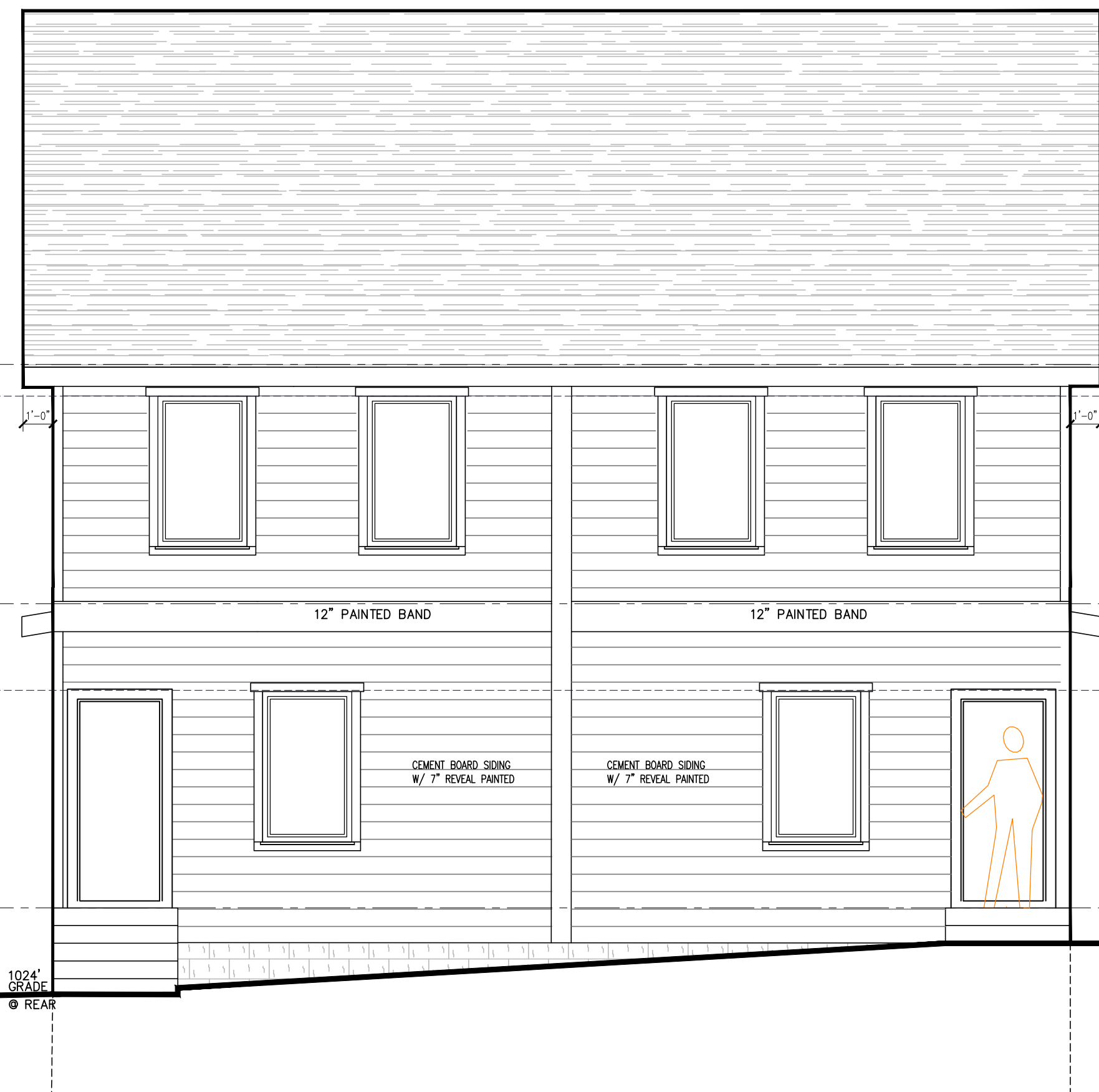
REAR ELEVATION UNIT "B" UNIT "A" 1/4" = 1'-0"
