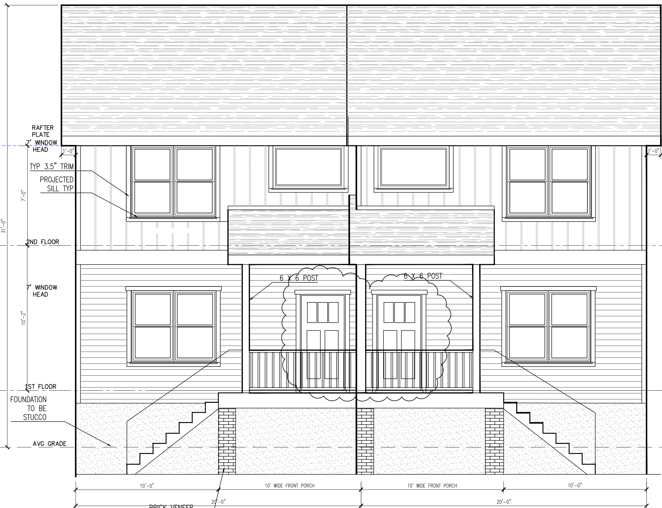
UNIT "B" FRONT ELEVATION
