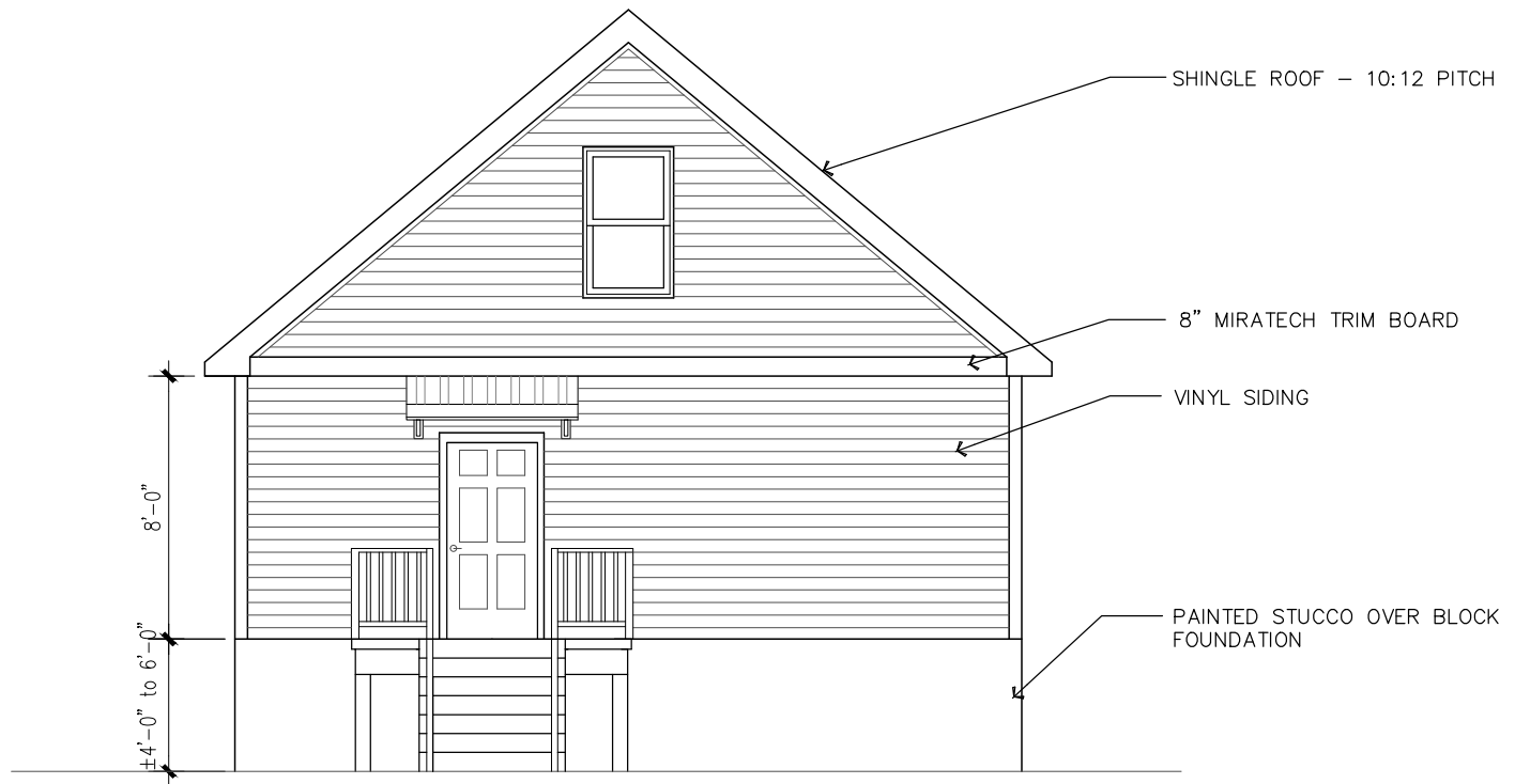
Rear Elevation 218 East Oldham Avenue 37917
