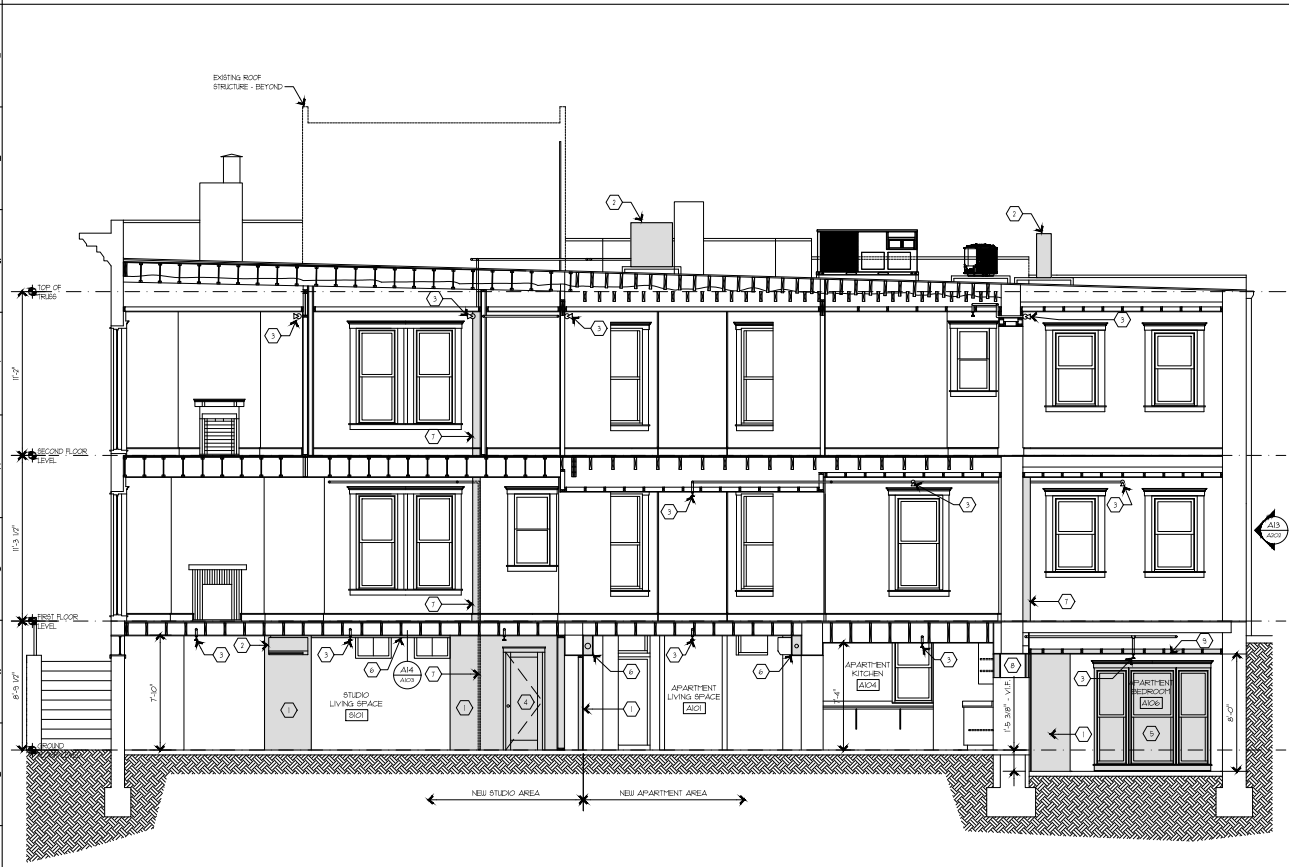
A1 BUILDING SECTION A203 1/8" = 1'-0"
