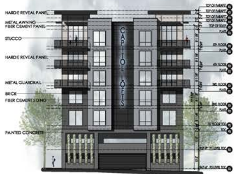
2 BLDG ELEVATION - EAST SCALE 1/16"=1'-0"
