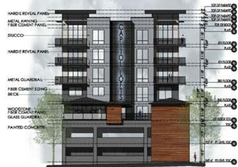
3 BLDG ELEVATION - WEST SCALE 1/16"=1'-0"
