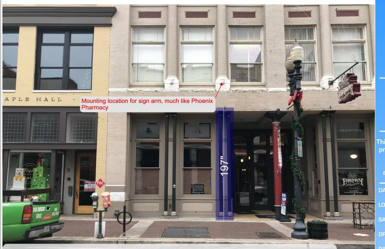
Drawing to represent that bottom of proposed sign will be approximately 197" to the sidewalk surface. Sign will install / mount much like the Phoenix Pharmacy sign to the right in this photo
