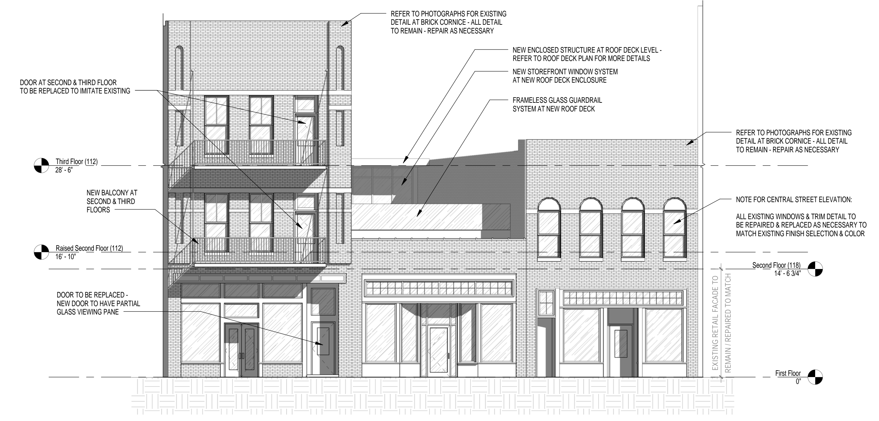
1 CENTRAL STREET ELEVATION 1/8" = 1'-0"
