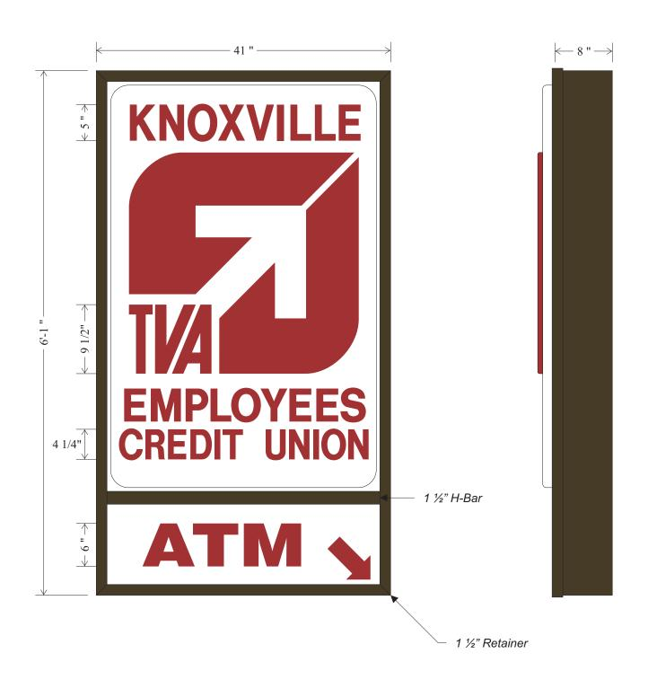
NOTE: One (1) single face wall sign with pan formed embossed acrylic faces painted on inside with acrylic paint. Internally illuminated with H.O. fluorescent lamps.
