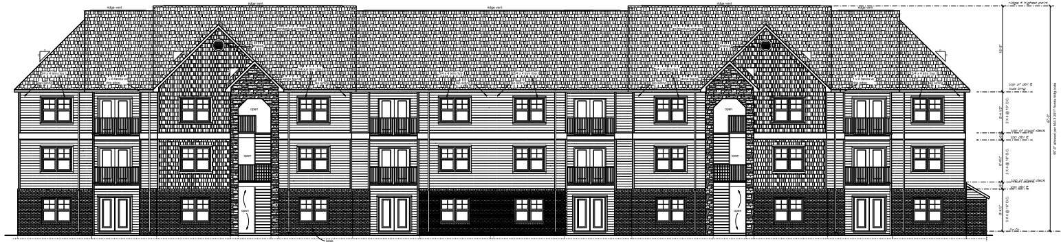
FRONT AND REAR ELEVATION - 2 BR 2 BATH DELUXE THREE STORY (24 UNIT) SC: 1/8"=1'0"
