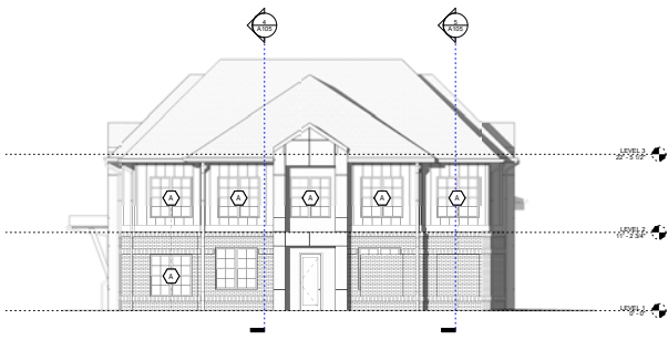
4 BUILDING ELEVATION - COMMUNITY BUILDING - SIDE ELEVATION 1/8" = 1'-0"
