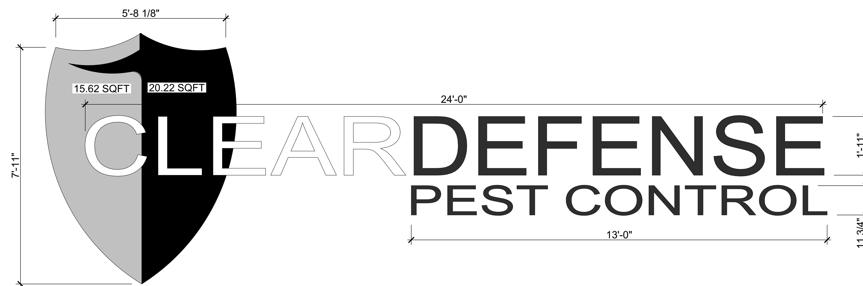
3 BUILDING SIGNAGE DETAIL SCALE: 1/2" = 1'-0"
