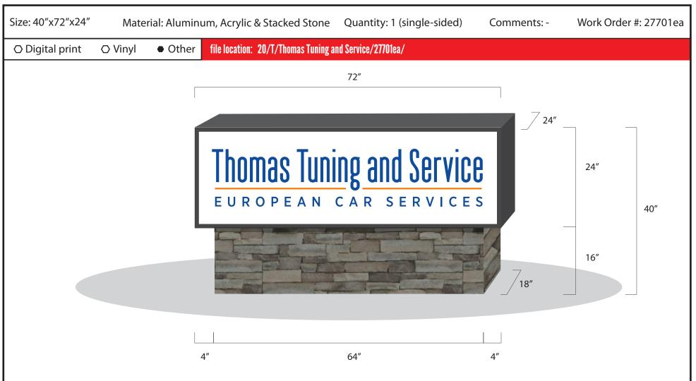
QTY 1 - Single-Sided Can Style Signage with Acrylic Face and Vinyl Lettering - Reinforced Stacked Stone Base - Internally LED Illuminated Sign Can
