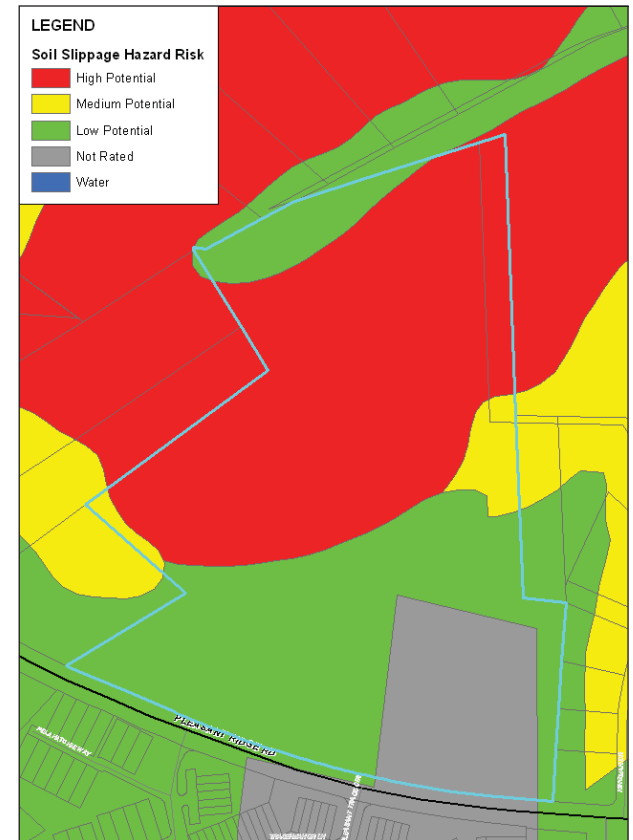
High slip potential soils are dominate in the failure area.
