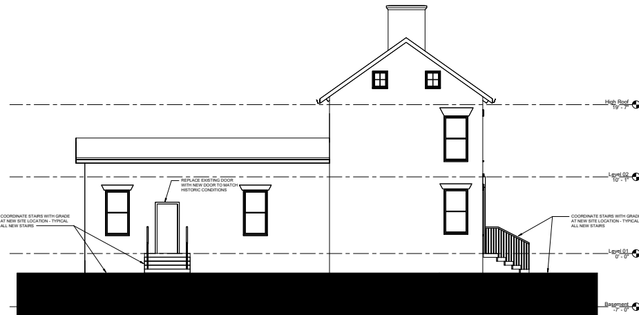
⊙ EAST BUILDING ELEVATION - NEW CONSTRUCTION 1/4" = 1'-0"
