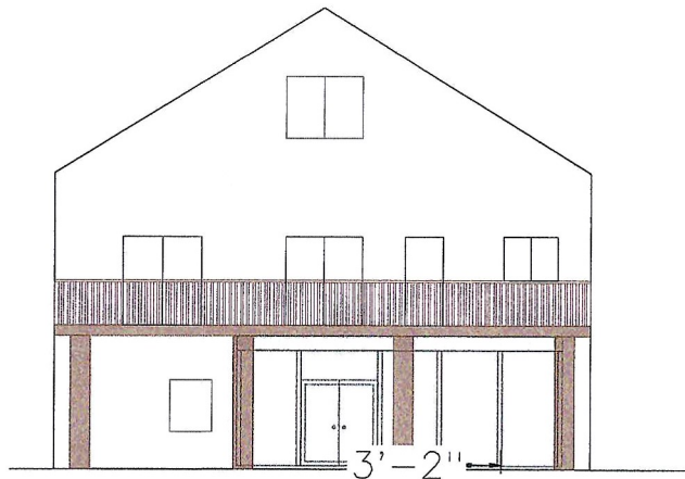
Rear Elevation w Sun Room - Glass enclosure under deck
