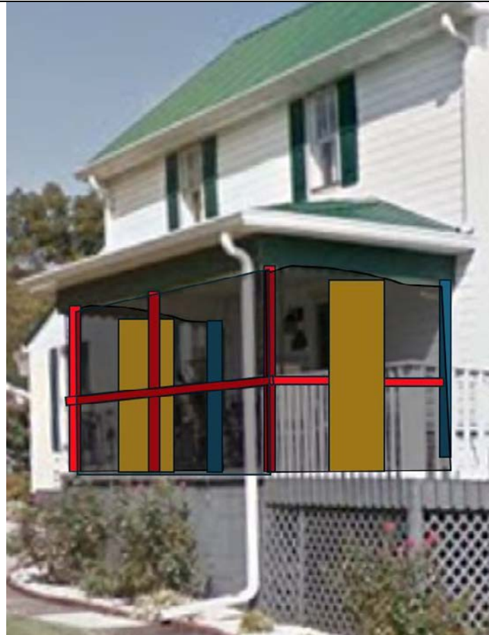
Image 2: Proposed Screening of Porch. Red – New posts / handrails Yellow – Doorways & supports Blue – Existing exposed timber to be utilized.
