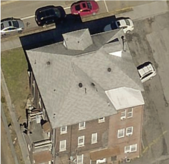
EXISTING ROOF TO BE REBUILT TO PROVIDE TALLER CEILING ON THIRD FLOOR
