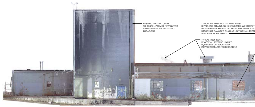
PARTIAL NORTH BUILDING ELEVATION - EXISTING 3 AD3.2 1/8" = 1'-0"
