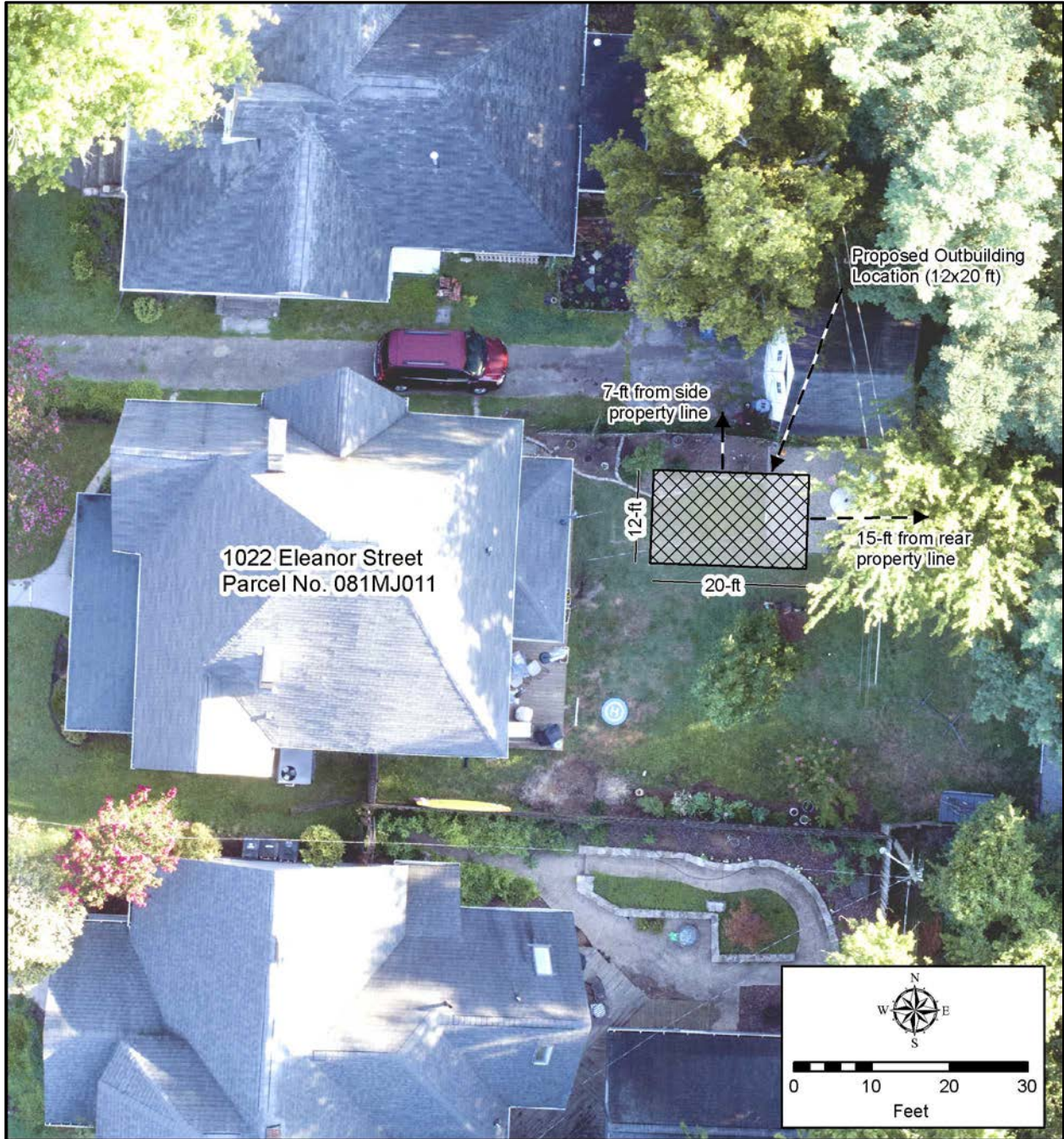
Figure 1. Plan view of the proposed 20x12-ft outbuilding location. Proposed outbuilding measures 7-ft from the north side property line and 15-ft from the rear (east) property line.
