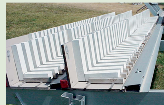
"L-Joint" visual appearance environmental test
