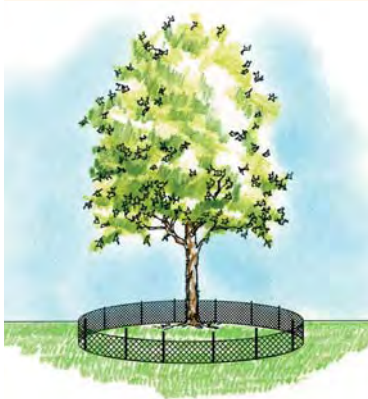
Figure 4. Protective silt fence located beyond tree's dripline.
